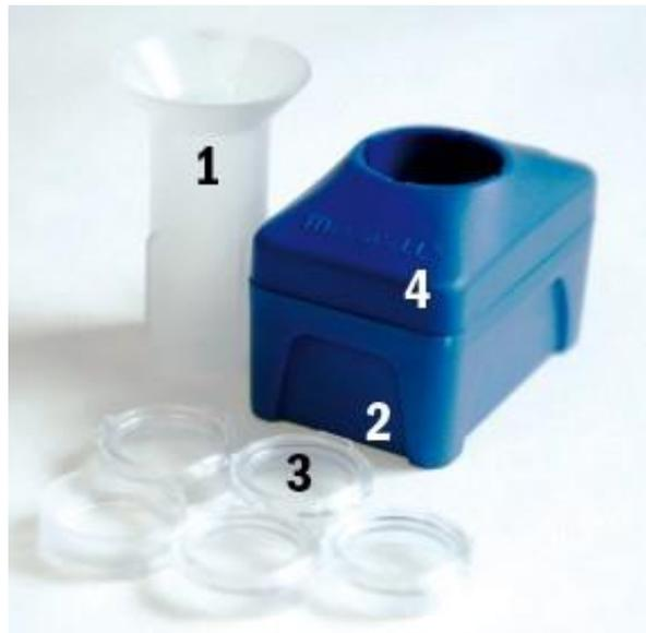
*MetaCell® separation tube consists of filling funnel (1), which is accompanied by a plastic ring (2) holding a separation membrane (3), the tube and ring complex are fixed in a flown blood reservoir (4).*
