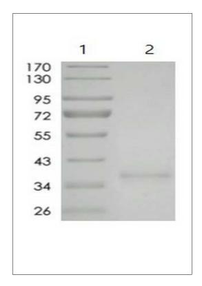
SDS-PAGE: Spike RBD protein run on a SDS-PAGE showing greater than 95% purity.
