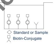
Following incubation unbound biotin-conjugated anti-Human IFN $\gamma$  antibody is removed during a wash step. Streptavidin-HRP is added and binds to the biotin-conjugated anti-Human IFN $\gamma$  antibody.
