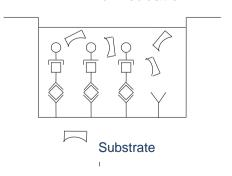
A coloured product is formed in proportion to the amount of Human IFN $\gamma$  present in the sample or standard. The reaction is terminated by addition of acid and absorbance is measured at 450 nm. A standard curve is prepared from 7 Human IFN $\gamma$  standard dilutions and Human IFN $\gamma$  sample concentration determined.
