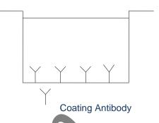
Human IFN $\gamma$  present in the sample or standard binds to antibodies adsorbed to the microwells. A biotin-conjugated anti-Human IFN $\gamma$  antibody is added and binds to Human IFN $\gamma$  captured by the first antibody.
