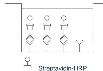
Following incubation unbound Streptavidin-HRP is removed during a wash step, and substrate solution reactive with HRP is added to the wells.
