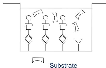
A coloured product is formed in proportion to the amount of human IL-17A present in the sample or standard. The reaction is terminated by addition of acid and absorbance is measured at 450 nm. A standard curve is prepared from 7 human IL-17A standard dilutions and human IL-17A sample concentration determined.
