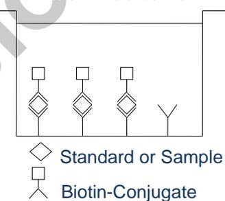
Following incubation unbound biotin-conjugated anti-human IL-5 antibody is removed during a wash step. Streptavidin-HRP is added and binds to the biotin-conjugated anti-human IL-5 antibody.
