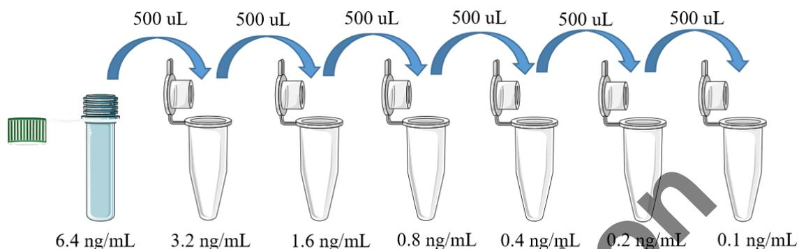
1×Assay buffer serves as the zero standard (0 ng/mL). The reconstituted standard stock should be aliquoted and stored at -20°C for up to one month. Avoid repeating freezing/thawing cycles. Please do not store the diluted standard solutions. It is recommended that the users establish their own dilution factors based on the concentration range of their samples.
